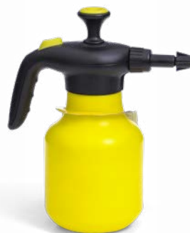
Pressure sprayer Type 3132* 1 or 1.5 liter sprayer for plant protection products, with a 2-in-1 valve that enables automatic pressure release in case of overpressure and manual pressure release, if required. Also available as a 360° sprayer.
