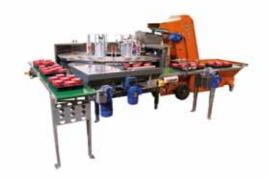
The latest development for filling pots in trays with soil. With its unique transportation system, the Javo Matrix offers a high output of trays per hour and a uniform, high quality, and precise fill for each pot. It even is possible to process different, staggered patterns.
