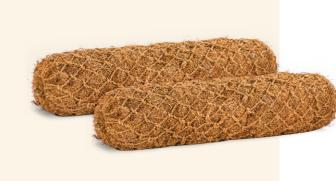
Bio logs consists of 100% coir fibre webs cross lapped, followed by needle punching or stich bonding. It collects and holds the grow medium providing a physically stable substance for root growth and gradually biodegrades for a sustaining erosion control system.
