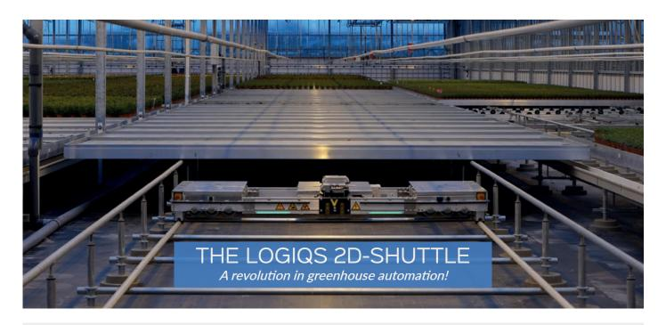
The 2D-Shuttle is the most efficient way of fully automating the growing area of the greenhouse while at the same time facilitating a fast and reliable transport flow of the mobile benches to and from the work area.
