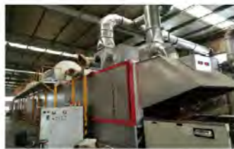
烘房本体保温使用多层专利结构, 烘房墙板采用三层绝热, 顶底板采用两层隔热结构; 减少能源消耗 Multi-layer structure wall board for less energy consumptions is offered with extra thicker boards within 150mm-220mm: 2-layer for top and bottom plate and 3-layer for oven body.
