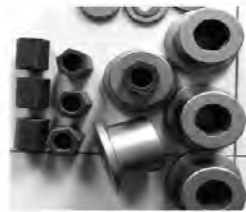
烘房花架输送链使用高强度链条, 每米增加到5只滚轮, 滚轮使用我公司专利产品: 耐磨无粉尘专用涂轮. Wickets conveyor using high strength chain, the roller (patented product) increased to 5pcs/meter; it has high wear resistance and dust-free.
