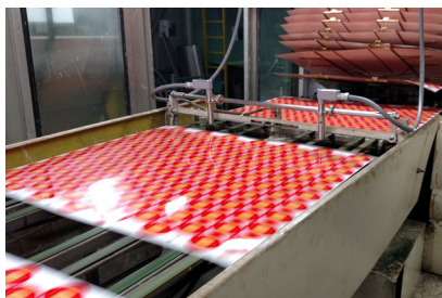
Rugged mounts and probe packages for fixed configurations with up to six probes
