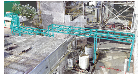
Point Cloud with Pipe Rack Concept/Tiddel
