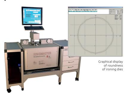
OEG GmbH provides high accurate optical measuring equipment for complete metrology of almost all tools for the beverage can manufacturing like ironing rings, punches, necking dies and knock outs.
