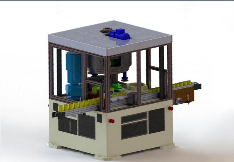
TIN CAN PARTING MACHINE Capacity: 400-450 can/min
