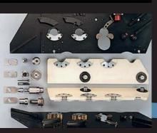
Complete sets of change parts for flanging and necking machines
