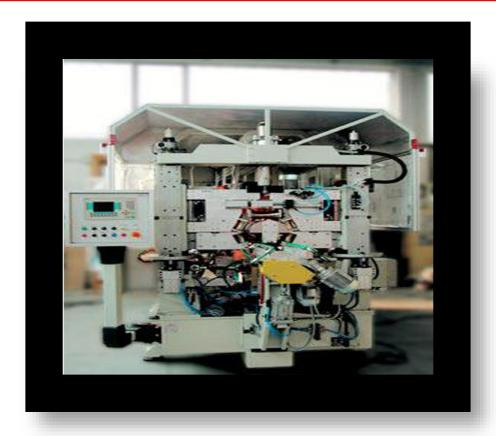
The automatic water heaters welder type C.S.A.B. for the longitudinal welding of internal body of water heaters and other purpose containers is designed and manufactured by GS&T. This machine features the possibility to roll form the steel body and immediately transfer it to the integrated welding station and weld it.
