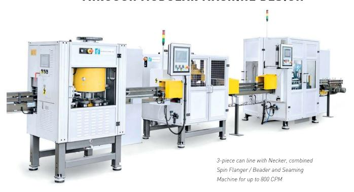
The modular design of the machines from GERMANN + FREI can be combined as desired and covers the entire backend in the manufacturing of 3-piece cans. From parting to can seaming, GERMANN + FREI builds machines that are known for their high reliability and smooth, running. The gentle handling of the cans is valued equally by customers in the milk powder and food industries – highest machine efficiency with easy handling.
