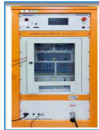
10KV Surge Generator
