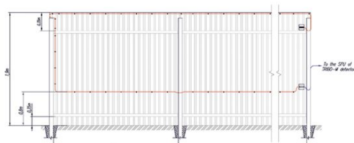
SENSITIVE ELEMENT LAYOUT ON WOODEN FENCE
