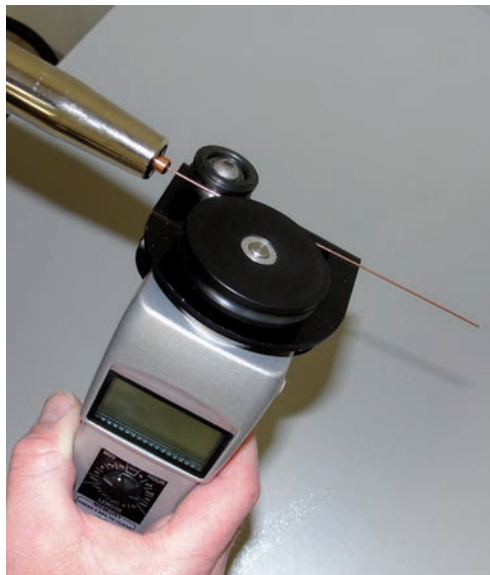
HHSS-12 obtaining measurement at the torch end
