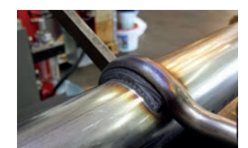
HD-MAG welding process
