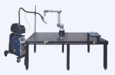
**Power Supplies:** TIG: Böhler (cold wire) water cooled: 320A AC/DC TIG: Böhler (cold wire) water cooled: 400A AC/DC
