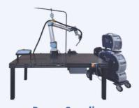
**Power Supplies:** MIG / MAG: Böhler water cooled 320A MIG / MAG: Böhler water cooled 400A MIG / MAG: Böhler water cooled 500A
