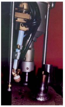
special torch for header drum stud welding
