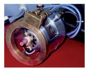
double gas shield chamber, liquid cooled
