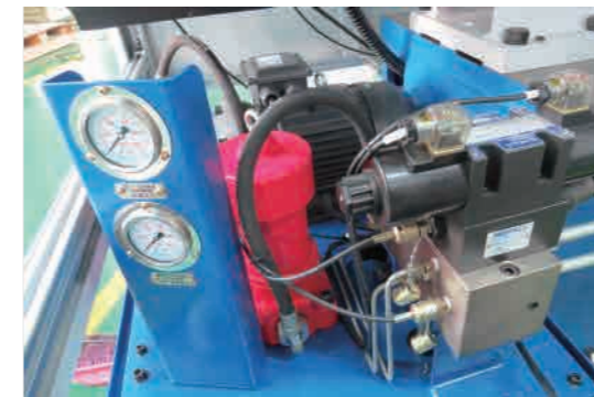
Oil temperature control system
