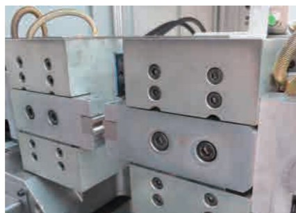
High accuracy self centering synchronous clamping system
