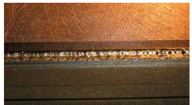
Welded seam executed with EBO Jump technology
