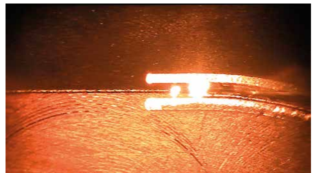
Simultaneous EB processing with pre-heating to the required temperature, welding and fully finished seam
