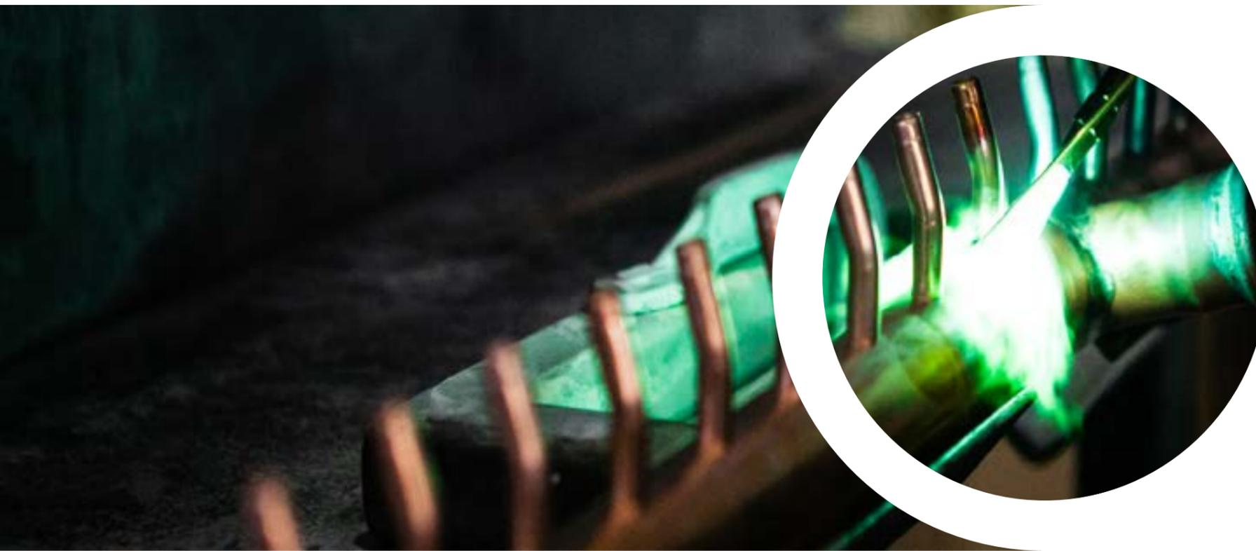
Various heating methods can be used to heat the filler material depending, in part, on the material in question: torch brazing, electric heating, vacuum or controlled-atmosphere furnace brazing.
