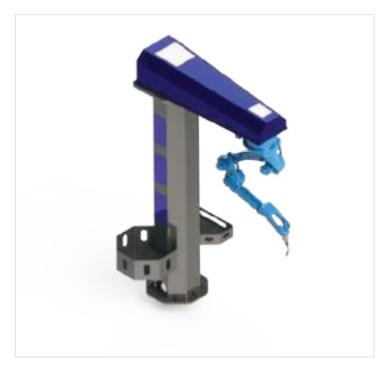
C-FRAME, fixed to the position of the robot relative to the workpiece. It is manufactured by being determined in special dimensions. this arm provides better access to the workpiece and helps to weld larger workpieces. makes it more efficient. The C-Frame is mounted directly on the floor or slider.
