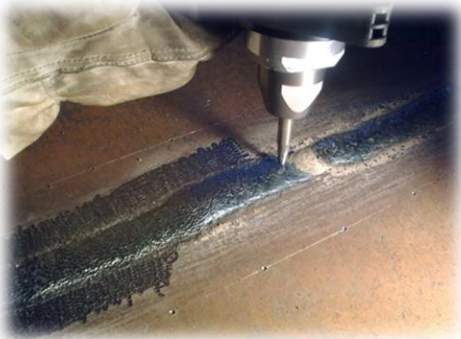
flat PIT treatment of complete weld including HEZ prevention of fatigue and stress corrosion cracking (SCC)
