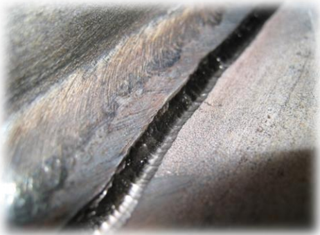
flat PIT treatment of complete weld including HEZ prevention of fatigue and stress corrosion cracking (SCC)
