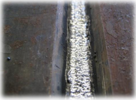
flat PIT treatment of every layer to avoid shrinkage and distorsion
