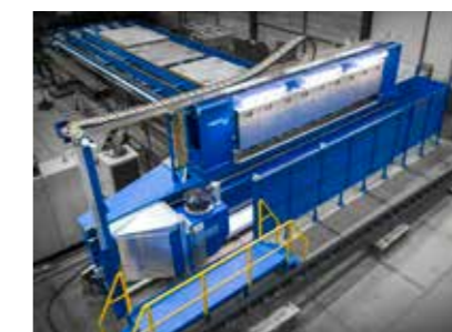
▲ PEMA EB for edge beveling.
