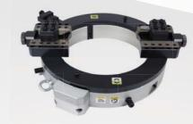
This is our new machine, stationary ring made by aluminum. Steel where strength is needed, aluminum where strength is less critical than weight.
