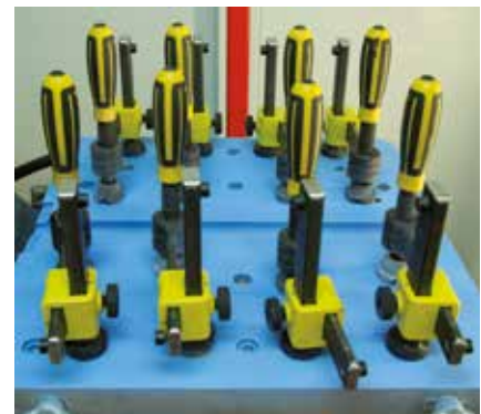
Welding fixture with ceramic coating
