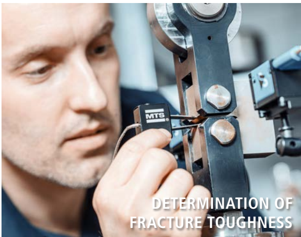
C(T) SPECIMEN ACCORDING TO ASTM E1820
