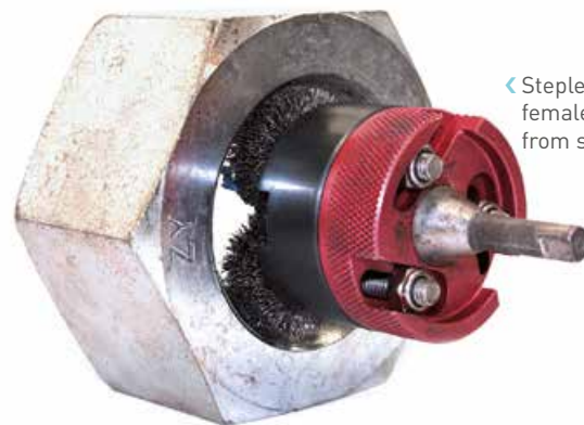
◀ Cleaner for external threads with automatic thread adjustment
