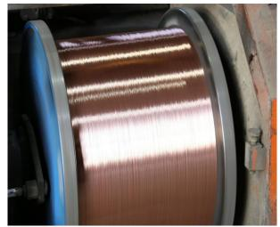
In this production step the attention of the qualified operators is critical. The wire produced after this process is sent to spooling. Any imperfections here such as lack of coppering, tolerances in diameters of the wire must be noted by the operators which have the responsibility to isolate the "lower standard" material from the "quality" one.
