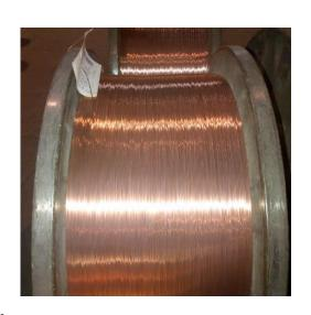
The wire once drawn to the "semi-manufactured" size of 2.00mm is chemically treated to be copper (or bronze or eco) coated.
