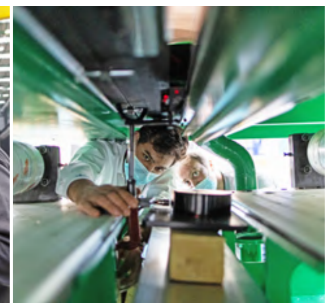
↑ Dimensional verification of the laser working spot
