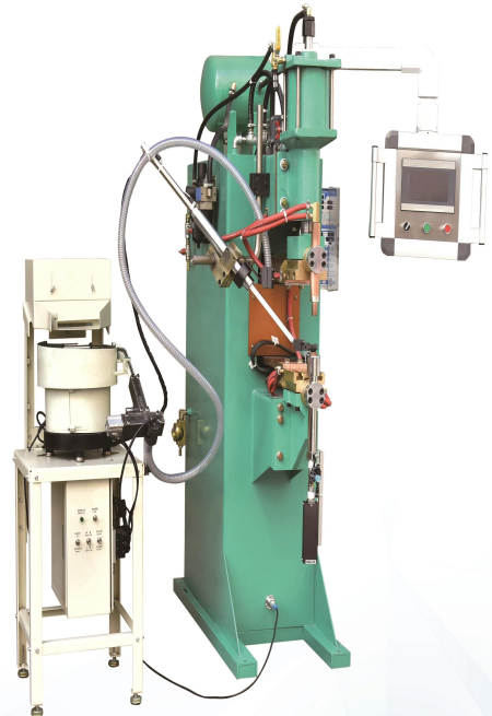
Spot Welding Machine & Nut Feeder
