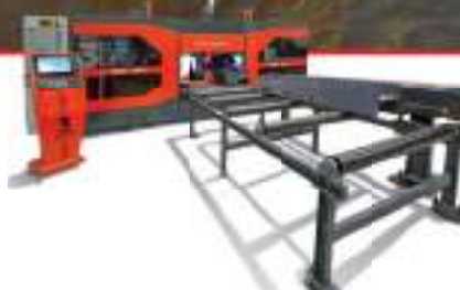
10-AXIS THREE-SPINDLE CNC DRILL LINE 10 EKSEN ÜÇ SPINDLE CNC DELİK DELME HATTI
